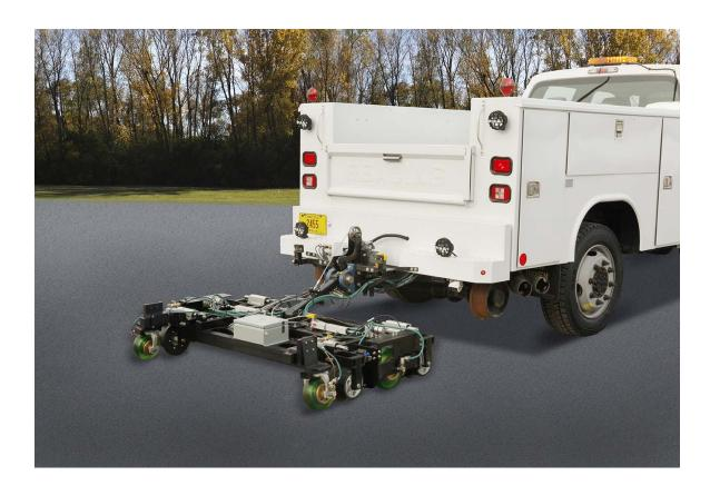
Nordco's is pleased to announce the new Flex rail flaw detection, featuring a hitch-mounted inspection carriage with patented XL9-11 wheel probes (including 11 inspection transducers), digital signal processing, and on-board Run-on-Run software.
